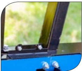
Track sweepers effectively remove sawdust from the bed rails
