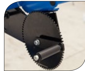
Manual head up and down system provides quick and exact head alignment
