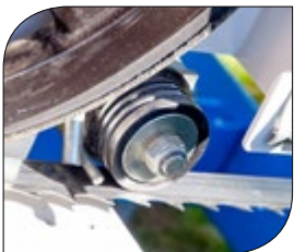
Blade guide rollers provide bigger quality of cutting
