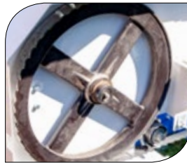
Pulleys adjustable in two directions
