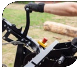
Easy-to-active clutch engagement provides right tension of the drive belt
