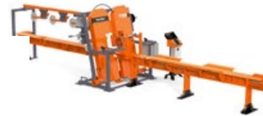
A typical layout consists of one or more TVS units which takes two sides off a log and then passes the two-sided cant on to the SVS (Single Vertical Saw). For those sawyers who want to produce four-sided cants from the log, we offer the TVS with a flat feed system which takes the two sided cant from the first TVS and removes two more sides in one pass.
