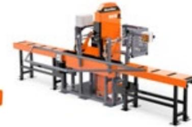
The SVS Single Vertical Saw simplifies the removal of the third side of a log during processing. Placed in the line behind the TVS, the SVS prepares the cant to move on to the resaw. The SVS has a maximum cut width of 300mm. The maximum material size is 400mm wide by 250mm high.
