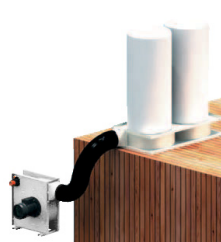
301-007 Chip Extraction System for Chip Containers Complete extraction system that includes filter, cyclone and chip collection bags. For use with a chip container. Delivery hose between cyclone and fan allows the fan to be located away from the cyclone system. Collection bag size is 2 x 250 litres. (for MP260 and MP160)
