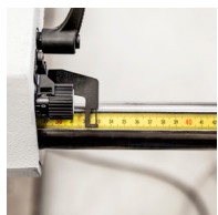
Board Fence Adjustable to tenths of a millimetre.
