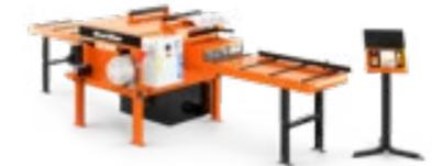
EG300 Multi-Rip Edger standardizes up to three board sizes for maximum timber recovery. The EG300 is the ideal companion for the Wood-Mizer Industrial SLP line. This machine comes standard with two blades (one moveable). Up to three additional blades can be added for full function Multi-Rip capability.
