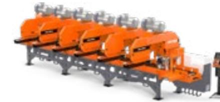
Ideal for companies that need a large capacity, heavy-duty multi-head resaw, the HR700's modular design makes it easy to expand from one to a maximum of six heads as their demands change. In its maximum six head configuration, the HR700 converts large cants into six boards and one slab in one pass.
