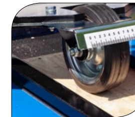
Hold-down rollers keep the boards straight during edging
