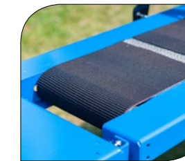
Power-feed tables with a speed of 9 m/min.
