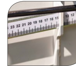
Scale indicates distance between blades with 1 mm accuracy
