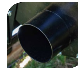
Sawdust collection with port to dust extraction system
