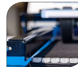
A removable board fence makes it easy to trim boards that already have one straight side
