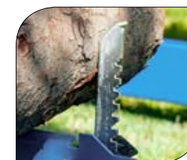
Quick-set log rests can be adjusted by hand
